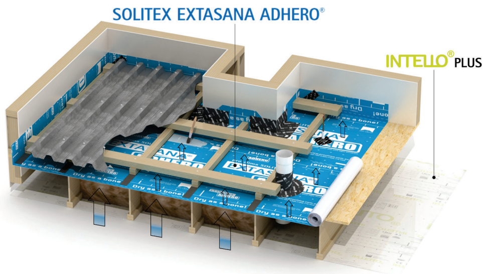
Figure 11. Typical ventilated low-pitch roof construction (Recommended)
