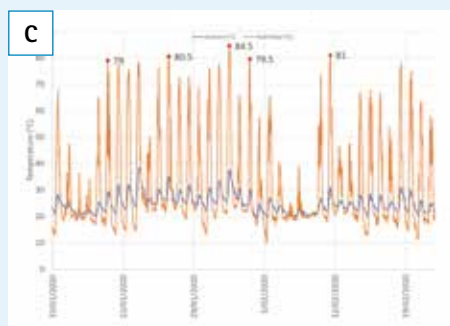
Figure 7.68: Roof Temperature measured in Sydney, January 2020 [111]. The blue line is the outdoor ambient temperature and the orange line is the roof surface temperature.
