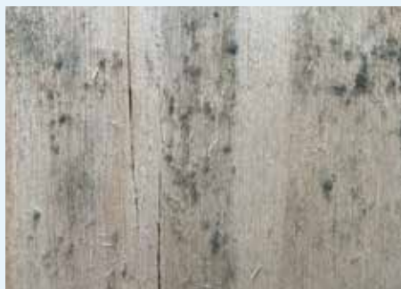
Figure 5.9: MI = 3, Visual findings of mould on surface, &lt; 10 % coverage, or &lt; 50 % coverage of mould (microscope)
