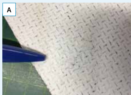
Figure 4.9: Early vapour permeable membrane technology utilising microporous membranes suffer from durability problems. A) 5 years of real aging and damages in the roofing membrane are already visible to the naked eye, B) the microscope reveals the cracks that lead to a lack of water tightness.
