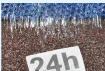
Figure 4.5: SOLID Acrylate adhesive used in pro clima TESCON EXTORA® is not water based in manufacture, i.e. there are no emulsifiers used with the risk of re-emulsifying. The manufacture is free of water and therefore the glue is resistant to water and high humidity.
