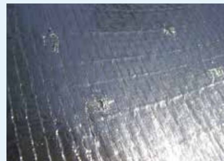
Figure 4.8: Perforations are often used to make a vapour barrier into a vapour permeable membrane. These can not be considered weatherproof as they do not meet the water barrier or air barrier properties necessary to provide weatherproofing necessary on the second line of defence and wind tightness required to enable the cladding to function effectively.
