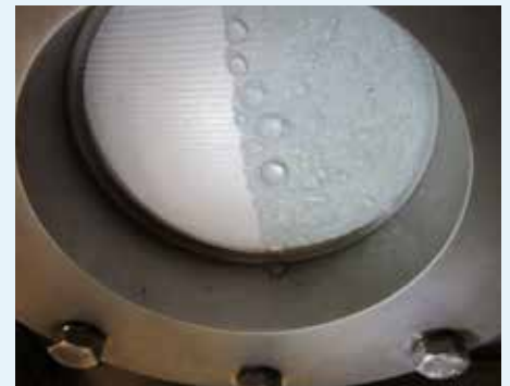
Figure 4.16: Microporous membrane when subject to surfactant such as oil, grease or timber tannins will allow water molecules to leak through the micropores. Left: oil applied to half the sample. Right: Leakage occurs through the microporous membrane half applied with oil.
