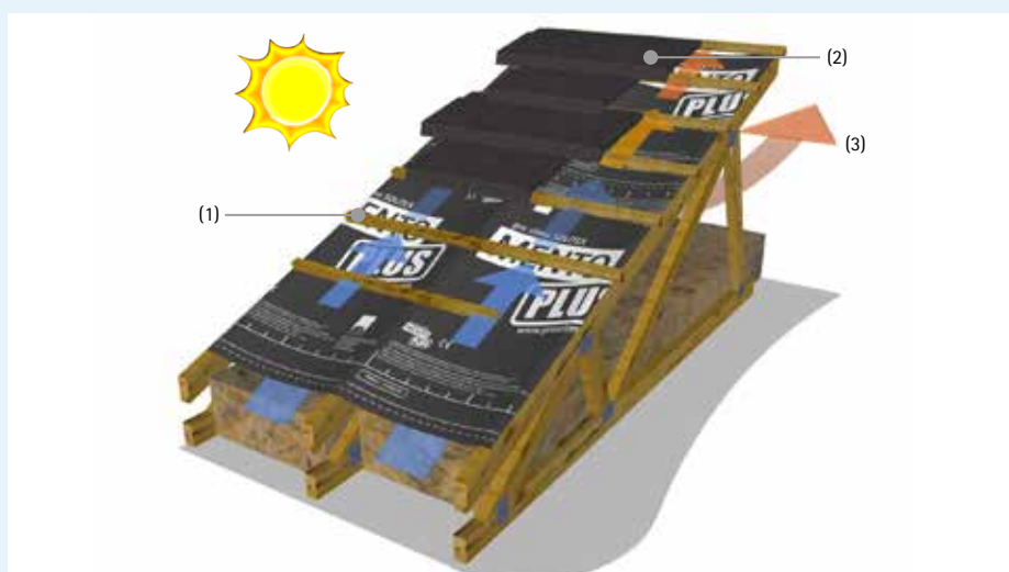
Figure 7.56: Tile roof have always allowed for incidental air flow under the battens and tiles, but not necessarily with dedicated inlet and outlet openings. (1) Fixing batten, (2) Roof tiles, (3) Attic Ventilation (opening to ceiling area ratio 1:300); Tile fixing methods has always achieved a ventilated cavity by default. The membrane under the battens allows for an airflow pathway that helps to remove heat by convection. The air layer means the membrane stays cooler than when pushed hard against a metal sheet cladding material.
