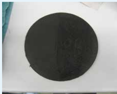
Figure 4.17: Non-microporous TEEE membrane when subject to surfactant such as oil, grease or timber tannins will remain water tight. Left: oil applied to half of the sample. Right: TEEE membrane remains unaffected.
