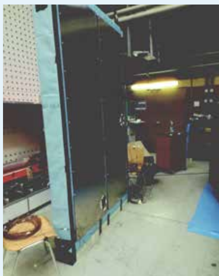
Figure 5.2c: The warm side before the mounting between the hot and cold box. [61]
