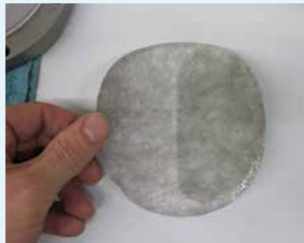
Figure 4.16: Microporous membrane when subject to surfactant such as oil, grease or timber tannins will allow water molecules to leak through the micropores. Left: oil applied to half the sample. Right: Leakage occurs through the microporous membrane half applied with oil.
