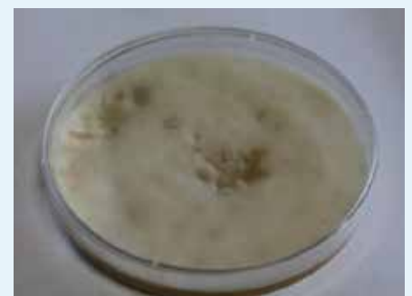
Figure 5.14: Sample scraped from the side of roof truss. Fungi identified from side of truss is penicillium. [69]
