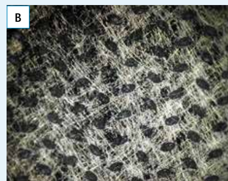
Figure 4.10: New generation technology utilising monolithic interlayers provide durable and reliable water barrier and air barrier properties for long term damage protection. 5 years of real aging, A) front side, B) back side.
