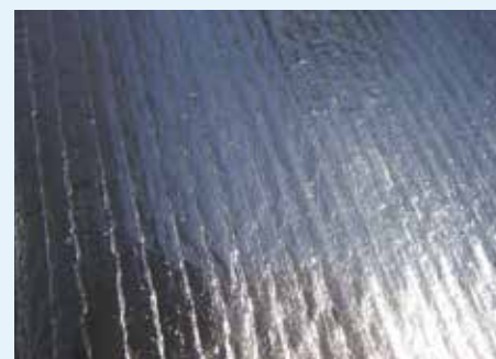
Figure 4.7: Vapour barriers usually contain a layer of aluminium foil. The foil itself is vapour impermeable and has no ability to allow structures to dry.
