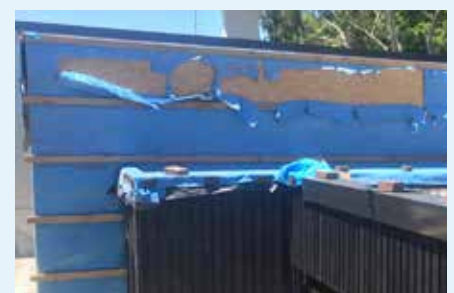
Figure 4.3: Left: Recently installed membrane. Right; Three months exposure, Sydney Australia.
