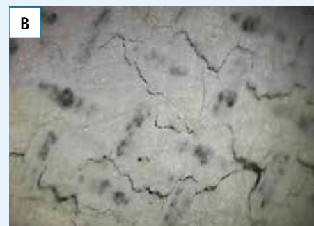
Figure 4.9: Early vapour permeable membrane technology utilising microporous membranes suffer from durability problems. A) 5 years of real aging and damages in the roofing membrane are already visible to the naked eye, B) the microscope reveals the cracks that lead to a lack of water tightness.
