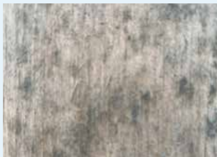
Figure 5.10: MI = 6, Heavy and tight growth, coverage about 100 %
