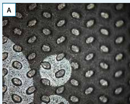
Figure 4.10: New generation technology utilising monolithic interlayers provide durable and reliable water barrier and air barrier properties for long term damage protection. 5 years of real aging, A) front side, B) back side.
