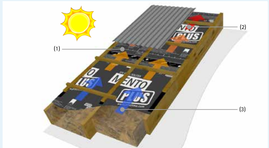
Figure 7.19: ASV is solar powered ventilation. Heat from the sun shining on the roof cladding, warms up the air beneath the cladding and induces a flow that moves the air upwards towards the ridge, while drawing in more air at the soffit. *Specific products may vary. Sun heats up roof cladding, (1) Heat transferred to air below, (2) Warm, buoyant air moves up the inclined air gap, (3) Cool air drawn in at eave
