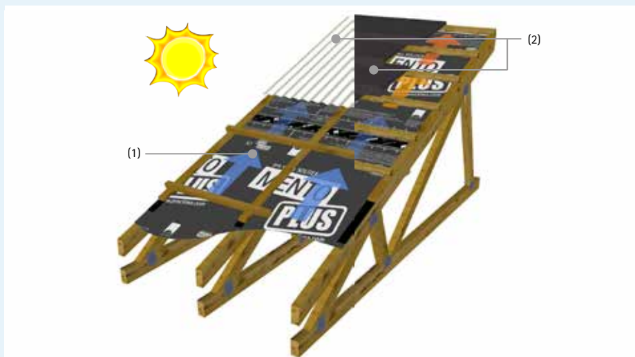
Figure 7.57: Purpose built air flow pathways allow heat to be removed before it reaches the insulation layers below. (1) Wind barrier creates an air cavity and chimney effect, (2) Shading (parasol) layer shades layers below from the sun
