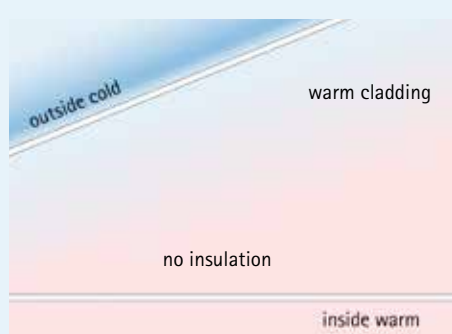
Figure 7.35: What used to be and what is now. Changing construction system dynamics due to insulation. Surfaces that were kept warm by energy inefficiency, such as immediately below the roofing materials (left) are now colder (right).
