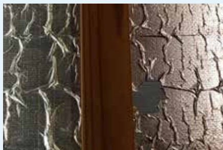
Figure 6.12: Lamination of materials with differing co-efficient of expansion/contraction under heat stress results in deterioration and ultimate delamination of the material layers. [71]
