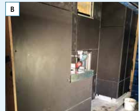
Figure 3.14: A full scale facade test of a drained and ventilated system with A) SOLITEX EXTASANA® WRB and B) Fibre cement cladding with a cavity, lan Bennie and Associates, Melbourne, Australia.
