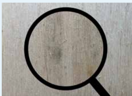
Figure 5.8: MI = 2, Several local mould growth colonies on surface (microscope)
