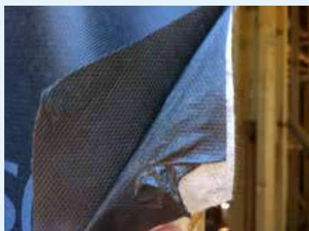
Figure 4.12: Thermoplastic Elastomer Ether Ester (TEEE) film is sandwiched between 2 protective fleeces.
