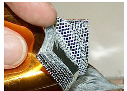
Figure 3: Low-emissivity surfaces are used in space where there is no atmosphere, and heat transfer is 100% radiative. (Hughes & Schaub, 2018)
