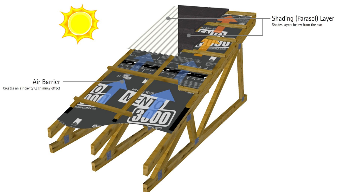
Figure 9: Purpose-Built airflow pathways allow heat to be removed before it reaches the insulation layers below.
