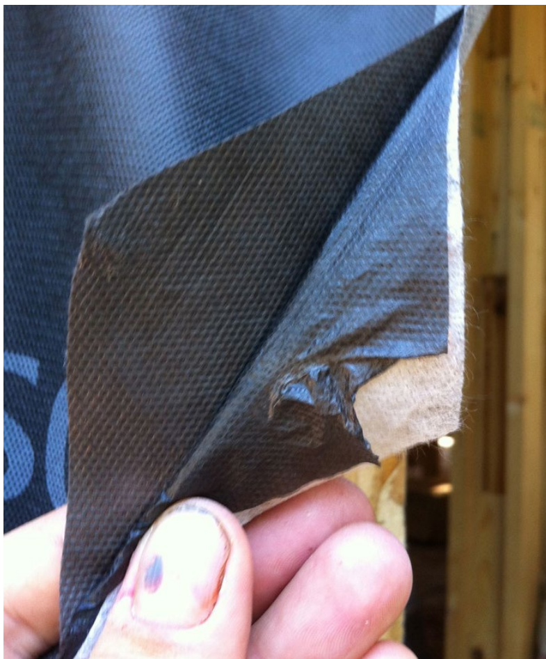
Showing the 3 layer build up of SOLITEX MENTO® (via BLDGTYP.com)
