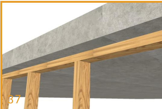
37 Soffit Junctions SOLITEX EXTASANA® should be connected into any concrete soffits that the framed wall butts into.
