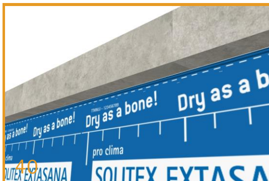
40 Weatherproof Seal Lay SOLITEX EXTASANA® overlap onto the ORCON® CLASSIC bead in full contact. DO NOT press the bead completely flat, allowing a lasting, flexible seal.
