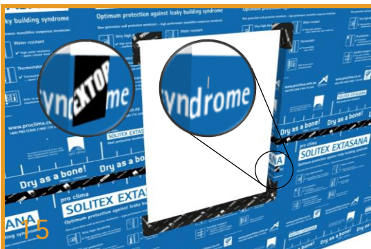
Seal Staples Using TESCON® EXTORA Staple holes around the window should be minimized. If any staples exist they should be covered with TESCON EXTOSEAL® or TESCON® EXTORA.
