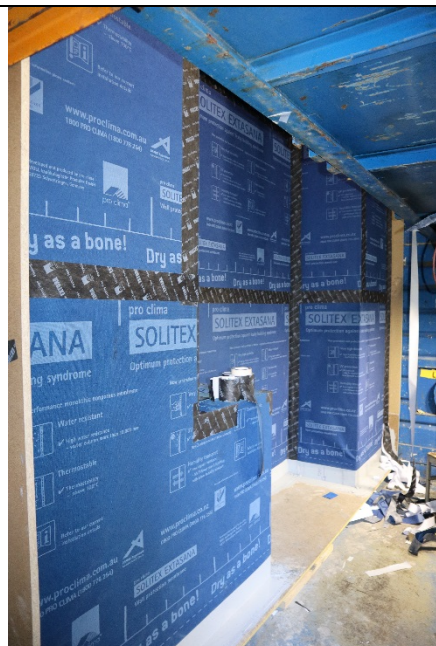
AS 4284 testing including pro clima SOLITEX EXTASANA® windtight & watertight weather resistive barrier, Ian Bennie & Associates, Melbourne Australia
