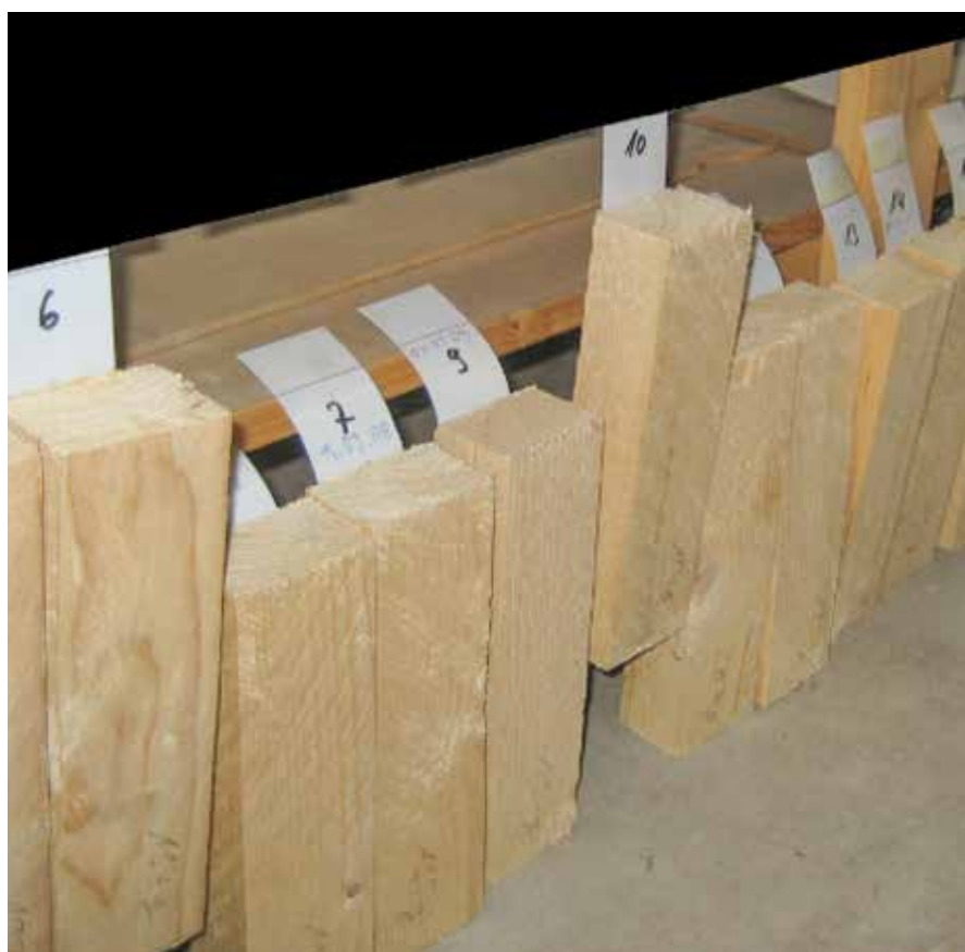
Cohesion adhesion test with 47 adhesive tapes: 40 adhesive tapes failed within two years in a long-term test with low loading.
