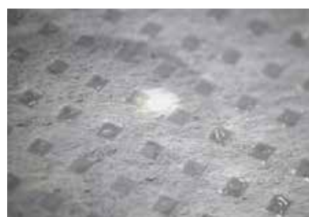
Double-layered airtightness membrane: Very good wetting and good adhesive ability, as the surface tension is greater than 45 \text{ N/mm} .
