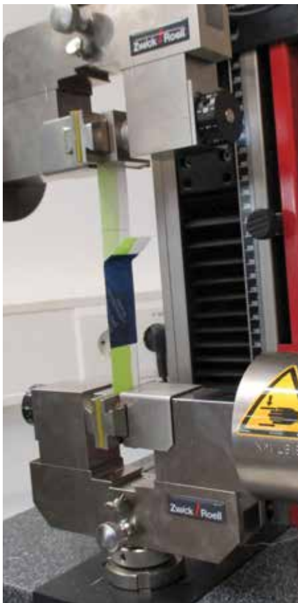
DIN 4108-11 specifies laboratory tests that have to be carried out for all adhesive tapes. This creates consistent quality standards and provide a basis for users to compare products.
