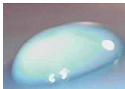
Weak wetting and poor adhesive ability for this PE airtightness membrane: approx. 35 \text{ N/mm}
